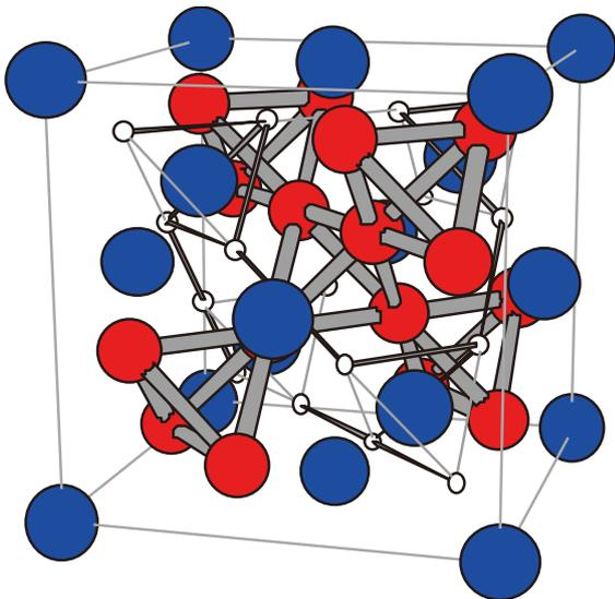
Fig. 1 Crystal structure of  $YMn_2$ , where Y and Mn atoms are indicated by blue and red circles, respectively. Small open circles show 16c sites where hydrogen atoms are located in hydrates, which are presumed to be occupied by implanted muons. These Mn atoms form a network of corner-shared tetrahedra known as a “pyrochlore” lattice.
