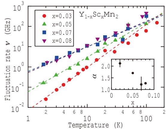
Fig. 2 Spin fluctuation rate ( $\nu$ ) as a function of temperature and Sc content ( $x$ ) in  $Y_{1-x}Sc_xMn_2$ . Solid lines are the results of curve fitting using a power-law ( $\nu \propto T^\alpha$ ). Inset:  $\alpha$  obtained by curve fits vs  $x$ .
